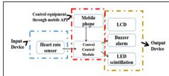
**Fig 3. A case of hardware composition of the Heart Monitoring System designed and make by student.**
