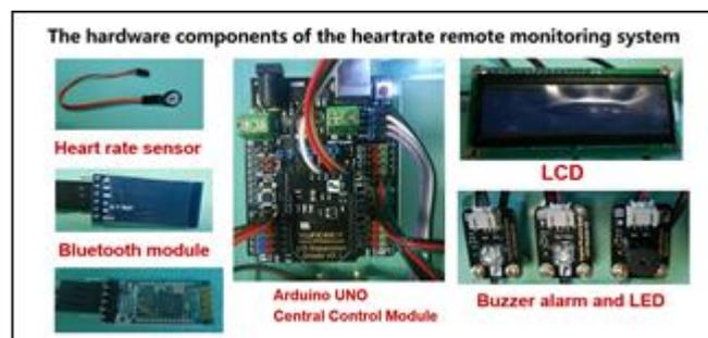
**Fig 4. The hardware components of a case of heartrate remote monitoring system, it would be selectly used by students themselves depend on their designed system functions.**
