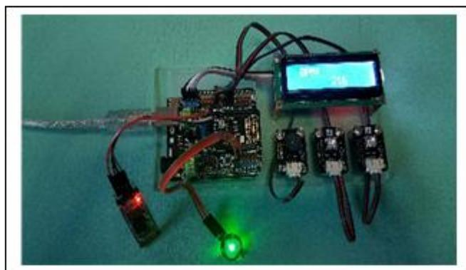
Fig 7. A case of the hardware system of the heartrate remote monitoring system the students build.
